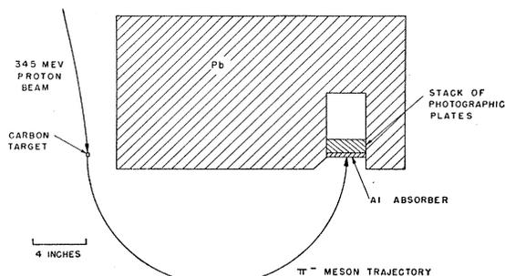
FIG. 1. Schematic diagram of apparatus for exposing plates.
