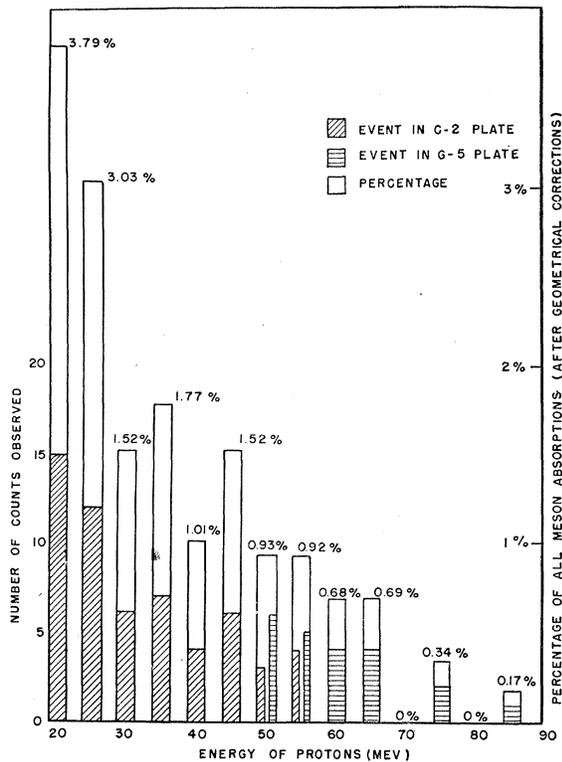
FIG. 4. Energy spectrum of emitted protons of energy greater than 20 Mev, before and after geometrical corrections.
