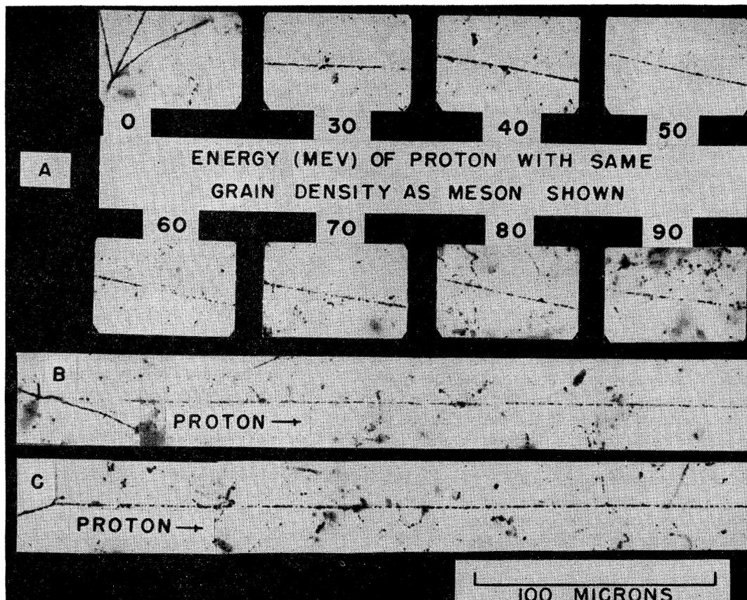
FIG. 2. (A) Photomicrograph of meson track taken at various velocities in G-5 plate. A proton at the same velocities would have the grain densities and energies shown. (B) 4-prong meson star, one of whose prongs is a 58-Mev proton. (C) Meson star with single prong, a 55-Mev proton. An electron is also associated with this event.
