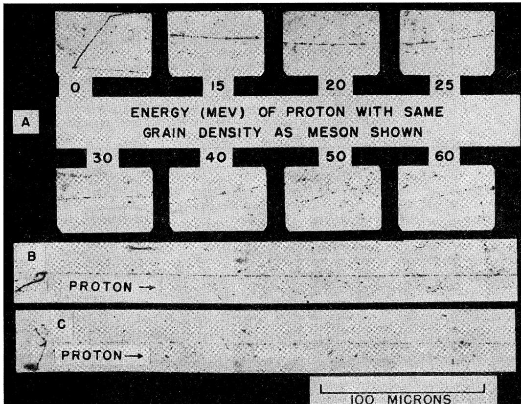
FIG. 3. (A) Photomicrograph of meson track taken at various velocities in a C-2 plate. A proton at the same velocities would have the grain densities and energies shown. (B) 2-prong meson star, one of whose prongs is a  $20\frac{1}{2}$ -Mev proton. (C) 3-prong meson star, one of whose prongs is a  $56\frac{1}{2}$ -Mev proton.
