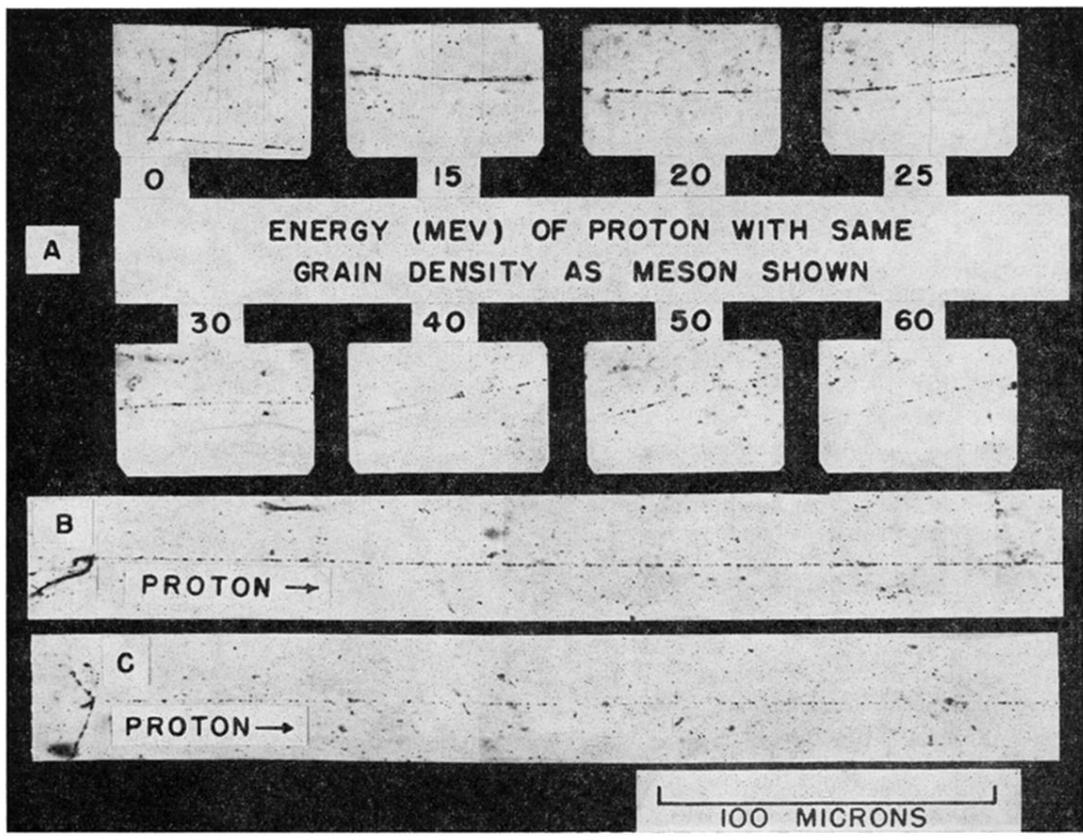
FIG. 3. (A) Photomicrograph of meson track taken at various velocities in a C-2 plate. A proton at the same velocities would have the grain densities and energies shown. (B) 2-prong meson star, one of whose prongs is a 20½-Mev proton. (C) 3-prong meson star, one of whose prongs is a 56½-Mev proton.
