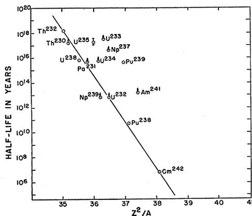
FIG. 1. Plot of spontaneous fission rates ( $\hat{\circ}$  signifies lower limit to half-life).
