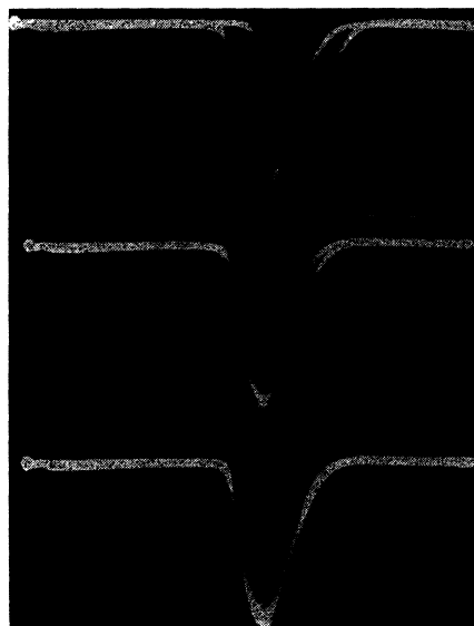
FIG. 4. Pulse matching. In the top picture the shift is 0.1 \mu\text{sec} , in the middle picture it is 0.02 \mu\text{sec} , and in the bottom picture the pulses are matched. The sweep is 2 \mu\text{sec} .
