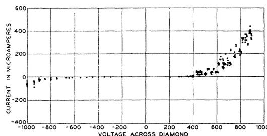
FIG. 2. High conduction in diamond. Dc current vs voltage.
