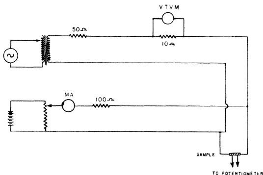
FIG. 1. Measuring circuit.
