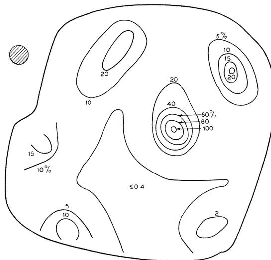
FIG. 4. Alpha-conduction in diamond. Counting efficiency inhomogeneities for electron pulses.
