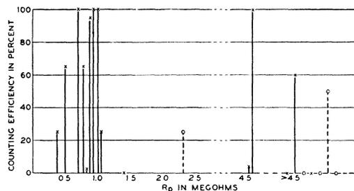
FIG. 5. Alpha-conduction in diamond. Counting efficiency vs equivalent parallel resistance. (X measured C.E., O estimated C.E.)
