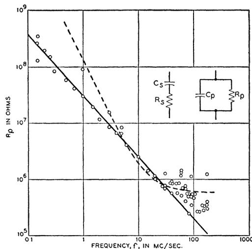
FIG. 1. Dielectric loss in diamond. Equivalent parallel resistance vs frequency of ac field.
