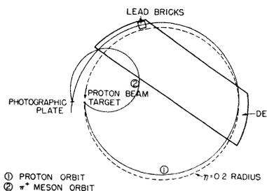
FIG. 3. Possible proton and  $\pi^+$  meson orbits in the fringing magnetic field.
