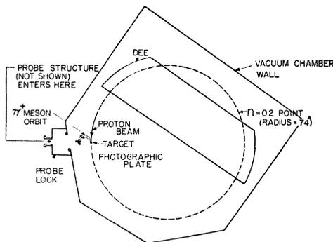
FIG. 1. Plan view of cyclotron showing  $\pi^+$  meson orbits.
