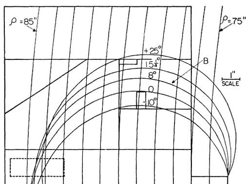
FIG. 5. Allowed and rejected orbits for 12-Mev  $\pi^+$  mesons. Mesons emitted at  $+25^\circ$  and  $-10^\circ$  with respect to the proton beam direction fail to pass through the opening of channel *B*.
