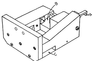
FIG. 4. Meson exposure chamber showing target *A*, channel *B*, and slot for plate holder *C*.
