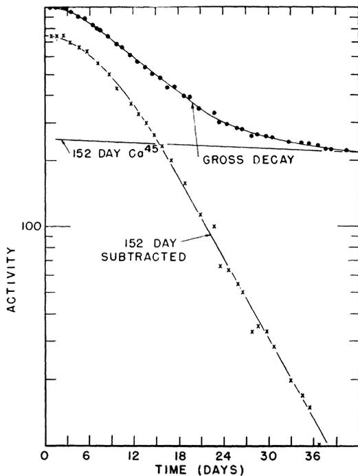
FIG. 1. Decay of calcium fraction separated from copper irradiated with 340-Mev protons.
