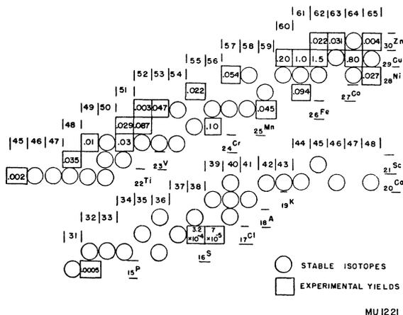
FIG. 4. Experimental yields from copper irradiated with 190-Mev deuterons. Yields are relative to Cu<sup>61</sup>.
