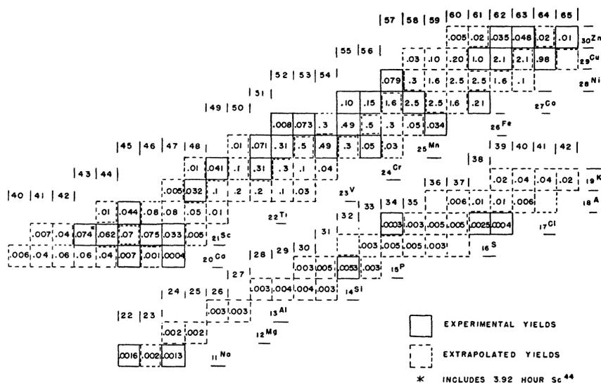
FIG. 6. Experimental, interpolated, and extrapolated yields from copper irradiated with 340-Mev protons. Yields are relative to  $\text{Cu}^{61}$ .
