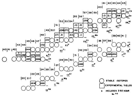
FIG. 3. Experimental yields from copper irradiated with 340-Mev protons. Yields are relative to Cu<sup>61</sup>.
