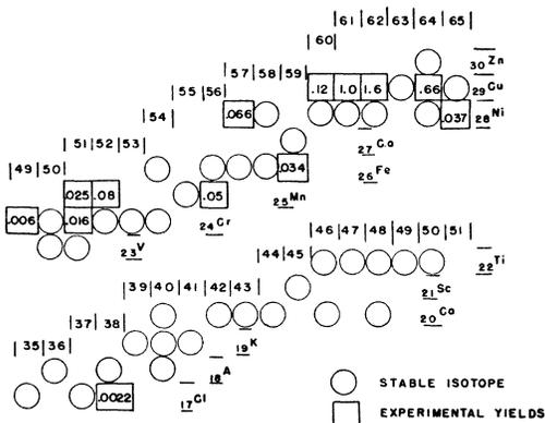
FIG. 5. Experimental yields from copper irradiated with 380-Mev helium ions. Yields are relative to Cu<sup>61</sup>.
