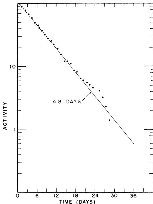
FIG. 2. Decay of calcium fraction separated from copper irradiated with 340-Mev protons counted through sufficient absorber to cut out the beta-particles of  $\text{Ca}^{45}$  and the  $\text{Sc}^{47}$  daughter.
