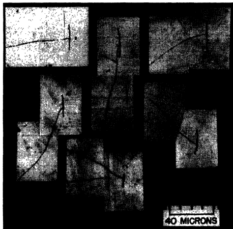
FIG. 1. Meson-induced fissions in uranyl acetate loaded G-5 emulsion (mostly plate 9876).
