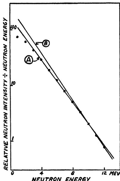
FIG. 1. Calculated distortion in a photographic plate spectrum from accepting tracks which start on the emulsion surface (having started in the paper wrapping). Line B is assumed to be the true spectrum. The dots indicate observed intensities; line A is the best line through the dots between 3 and 12 Mev. The slopes of lines A and B differ about 7 percent.
