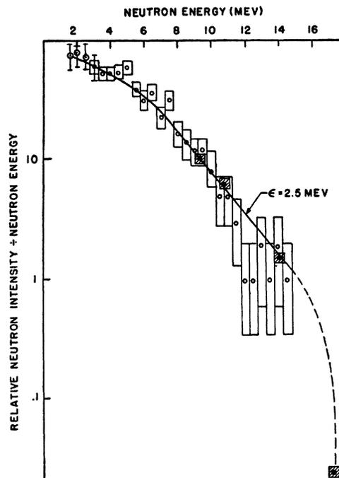
FIG. 2. Neutron energy spectrum at  $0^\circ$  from 15-Mev deuterons on beryllium. Open rectangles and points indicate photographic plate data, and cross-hatched squares are data from counter telescope. The data indicated by the open points (energies of 3 Mev and below) should be considered only indicative of the relative shape of the curve, as it is difficult to estimate the experimental error in this region. The solid line is the best straight line through the "constant" portion.
