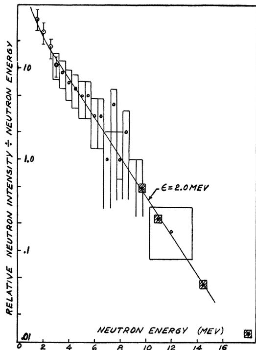
Fig. 5. Neutron energy spectrum at  $90^\circ$  from 15-Mev deuterons on aluminum. See Fig. 2 for explanation.
