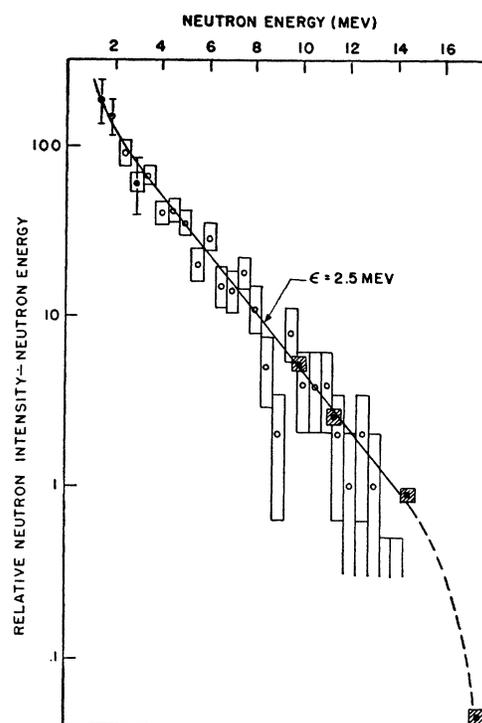
FIG. 4. Neutron energy spectrum at  $0^\circ$  from 15-Mev deuterons on cobalt. See Fig. 2 for explanation. A spectrum from copper and counter telescope spectra at  $20^\circ$  and  $45^\circ$  from cobalt agree within statistical errors.
