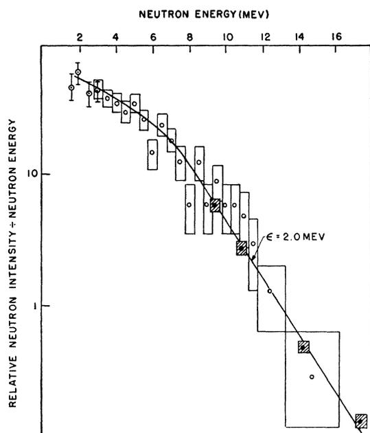
FIG. 3. Neutron energy spectrum at  $0^\circ$  from 15-Mev deuterons on aluminum. See Fig. 2 for explanation. A counter telescope spectrum at  $20^\circ$  agrees within statistical errors.
