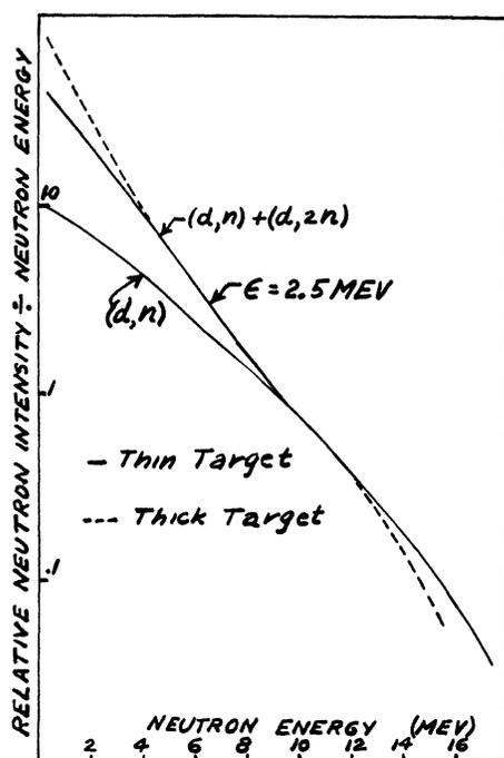
FIG. 7. Theoretical neutron spectrum to be expected from compound nucleus decay. Assumptions: Excitation energy = 20 Mev  $a$  [for use in Eq. (5)] = 3.6 Mev; binding energy of second neutron = 10 Mev.
