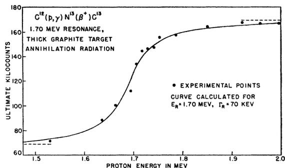
FIG. 2. Detail of the 1.70-Mev resonance. The curve is the integral of a single-level Breit-Wigner dispersion formula, taking into account the barrier for  $p$ -wave protons and other energy-dependent terms, assuming that  $E_R = 1.70$  Mev and  $\Gamma_R = 70$  kev.
