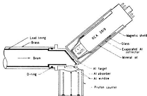
FIG. 2. Diagram of proton and gamma-ray counters.
