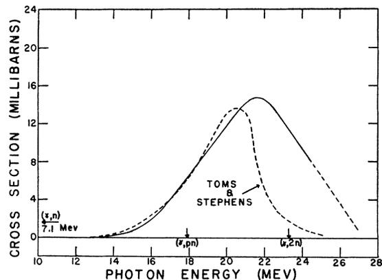
FIG. 3. Cross-section curves for the reaction  $Mg^{25}(\gamma, p)Na^{24}$ . The dotted line is the determination by Toms and Stephens. The arrows indicate thresholds for possible competing reactions.
