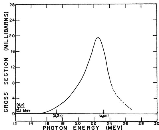
FIG. 4. Cross-section curve for the reaction  $Mg^{26}(\gamma, p)Na^{25}$ . The arrows indicate thresholds for possible competing reactions.
