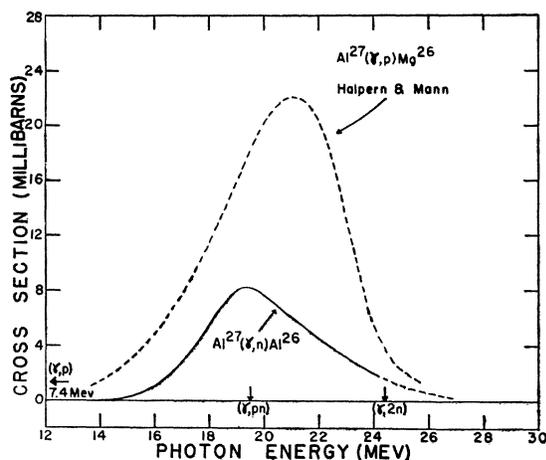
FIG. 1. Cross-section curves for the reactions  $\text{Al}^{27}(\gamma, n)\text{Al}^{26}$  (solid line) and  $\text{Al}^{27}(\gamma, p)\text{Mg}^{26}$  (dotted line, as measured by Halpern and Mann). The arrows indicate thresholds for possible competing reactions.
