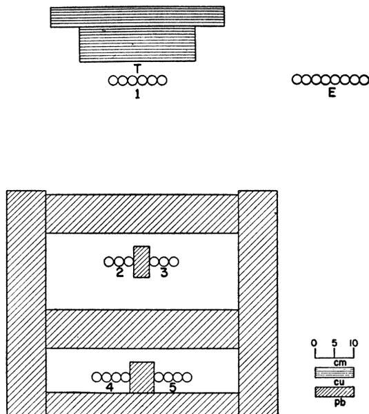
FIG. 1. Arrangement for observing penetrating showers.
