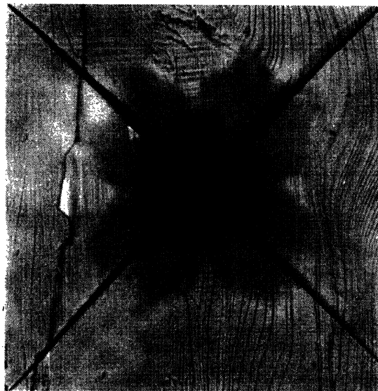
FIG. 13. Apparent cleavage of NaCl produced by punching on a cube face at room temperature, magnification 100\times .
