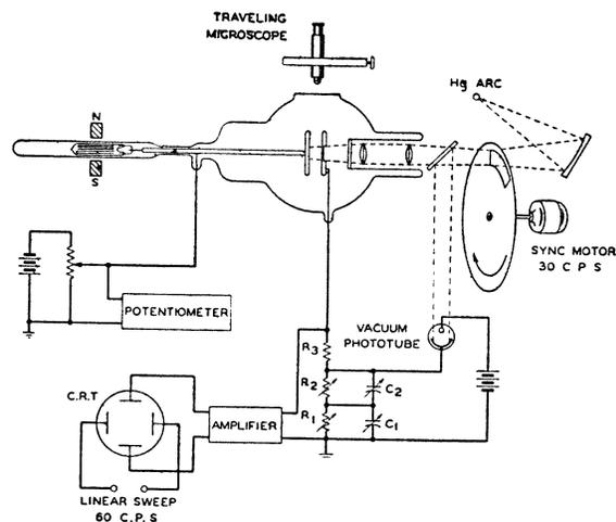
FIG. 3. Schematic diagram of arrangement of apparatus. The resistance of  $R_3$  is large compared with  $R_1 + R_2$ , so that the effect of the capacitance of  $C_1$  and  $C_2$  on the Townsend tube current is small. The horizontal sweep on the cathode-ray tube is operated at twice the disk frequency to provide a zero-line reference.
