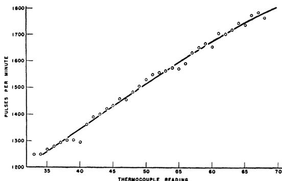
FIG. 6. Variation of the counting-rate with the temperature of the crystal. The warming and cooling rates were about  $15^{\circ}\text{C}$  per hour. Thirty-five divisions on the thermocouple scale approximately represent a temperature range of  $30^{\circ}\text{C}$ .
