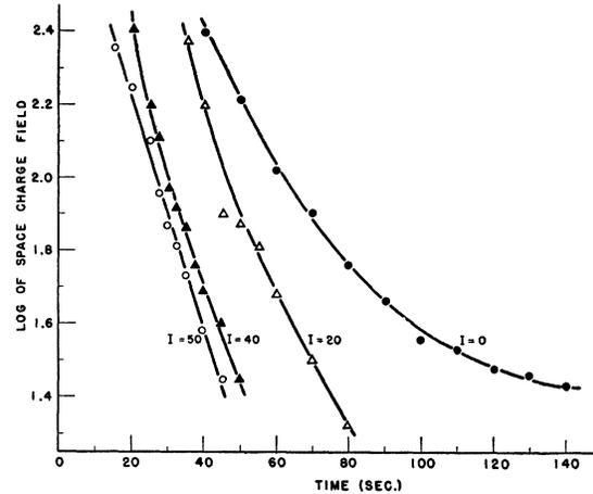
FIG. 3. Log plot of the decay of the space charge field with time for various intensities of illumination of the crystal. The intensity,  $I$ , is in arbitrary units.
