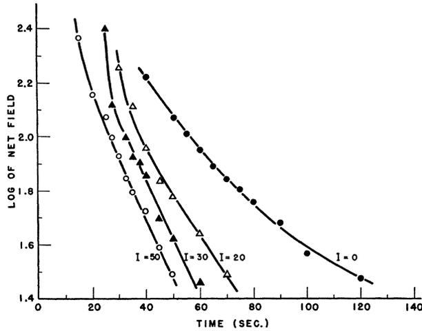
FIG. 4. Log plot of the decay of the net field with time for various intensities of illumination. The intensity  $I$ , is in arbitrary units.
