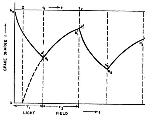
FIG. 2. Representation of the variation of the space charge field during the field-light cycle.
