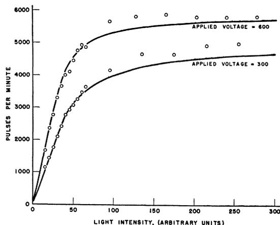
FIG. 5. Variation of the counting rate with the intensity of illumination during the field-light cycle. The full line shows the expected variation; the points plotted are those obtained experimentally.
