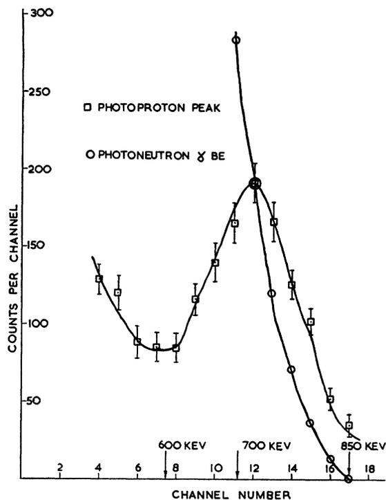
FIG. 1. Photoproton distribution from Na<sup>24</sup>  $\gamma$ -rays disintegrating deuterium in ion chamber; and deuterium recoils from RdTh- $\gamma$ -Be neutrons.
