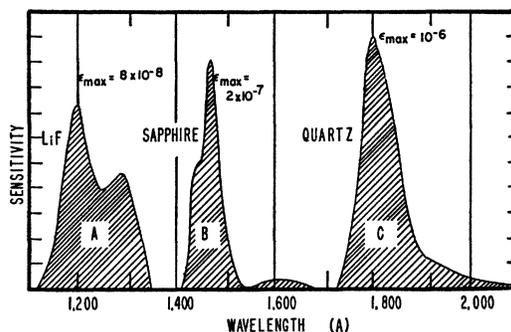
FIG. 3. Spectral response curves of three types of ultraviolet photon counters used in the rocket. The maximum photoelectron yields,  $\epsilon_{\text{max}}$ , for each tube are indicated in units of counts per quantum.
