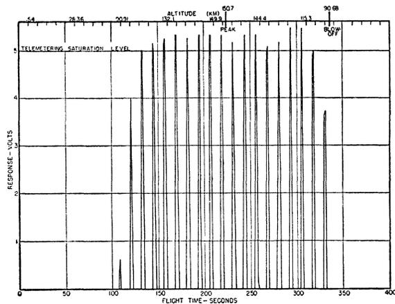
FIG. 1. A plot of data read directly from the telemetered record of the counting rate of an x-ray photon counter. The sharp responses occurred each time the spinning rocket presented the tube to the sun. The telemetered signals were not continuous, but the commutation rate was rapid enough to provide about eight points per exposure. In the illustration, smooth curves are drawn through the experimental points.
