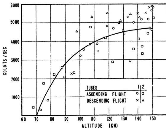
FIG. 2. Intensities measured with two nearly identical photon counters in the 1100A-1350A wavelength band. Four sets of points are plotted representing the telemetered data of the two tubes, corrected for saturation and effect of time constant, in ascending and descending portions of the rocket flight.
