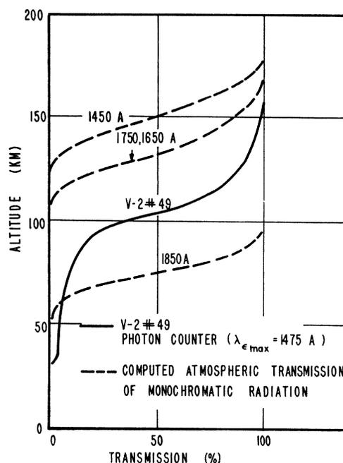
FIG. 5. Penetration of the atmosphere by ultraviolet radiation in the neighborhood of  $\lambda 1500\text{A}$ . The solid line is obtained from rocket measurements made with tube B of Fig. 3. The broken line curves were computed from absorption data of reference 5. Data for  $\lambda 1750$ , and  $\lambda 1650\text{A}$ , on either side of the absorption maximum at  $\lambda 1450\text{A}$ , almost coincide and are drawn as a single curve.
