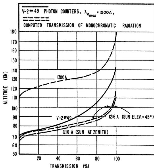
FIG. 4. Penetration of the atmosphere by ultraviolet radiation in the 1100A-1350A spectral region. The solid line is obtained from the data of two photon counters. The dashed line curves were computed from published absorption coefficients (references 4 and 5) at  $\lambda 1216\text{A}$  and  $\lambda 1300\text{A}$  for a sun elevation of 45 degrees. The dot-dash curve was computed for the sun at its zenith.
