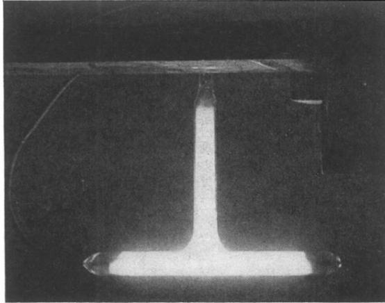
FIG. 1. Abrupt condenser discharge through a tube with side arm.
