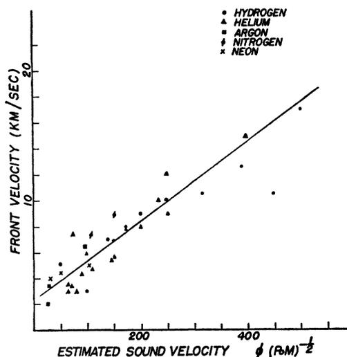
FIG. 3. Plot of front velocities of luminosity against an estimated sound velocity obtained by combination of capacitor potential (volts), initial gas pressure (mm Hg), and molecular weight.
