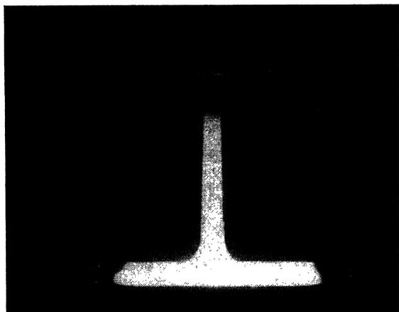
Fig. 1. Abrupt condenser discharge through a tube with side arm. Luminosity is sharply terminated by constriction.
