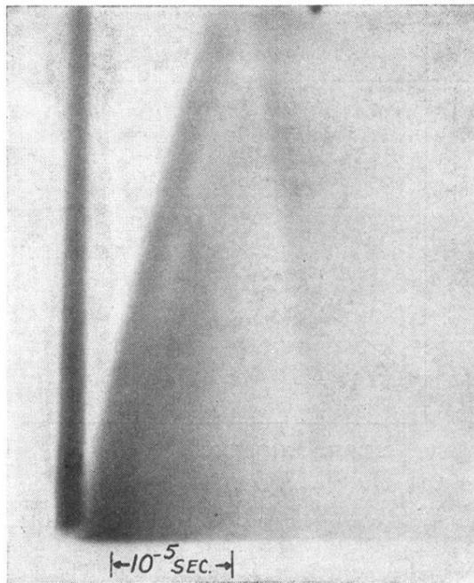
FIG. 2. Rotating mirror photograph of side arm of tube shown in Fig. 1. Stationary reference image at left. Lines parallel with stationary trace give instantaneous distributions of luminosity along side arm.
