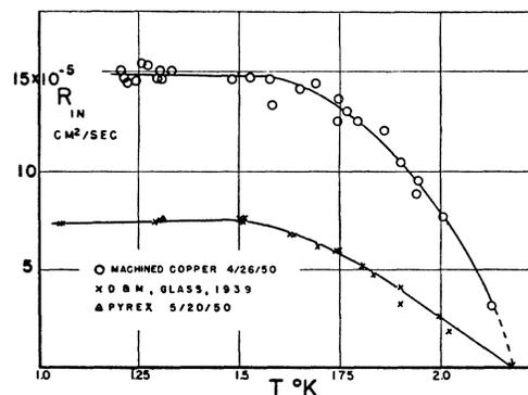
Fig. 7. HeII film transport rates over machined copper (typical curve).
