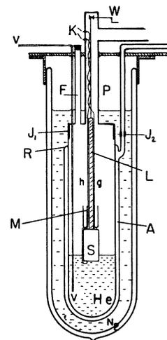
FIG. 3. Sectional view of the helium cryostat.
