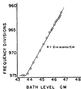
Fig. 4. Typical depth gauge calibration curve.
