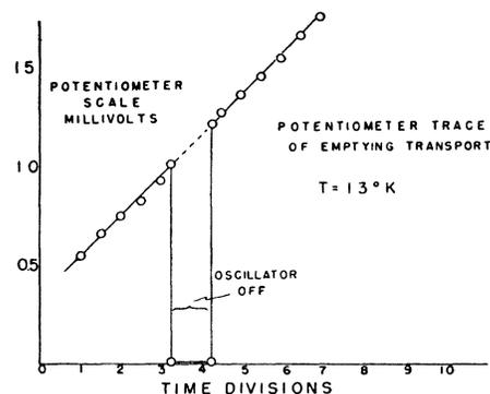
Fig. 5. Effect of capacitor excitation on transport rate.
