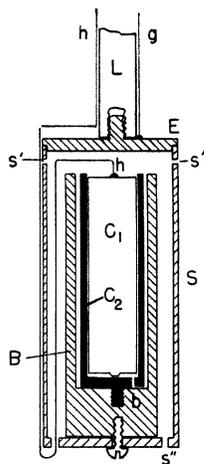
FIG. 1. Sectional view of container, depth gauge, and radiation shield assembly.
