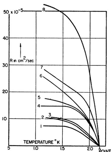
FIG. 11. HeII film transport rates for: (1) glass (D and M), (2) stainless steel, (3) iron, (4) machined copper, (5) lead, (6) burnished copper, (7) etched and oxidized copper, (8) etched copper (all drawn to the same scale).
