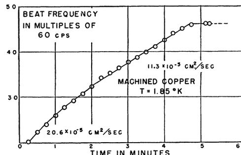
Fig. 6. Typical emptying curve for a machined copper container.
