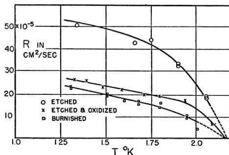
FIG. 8. HeII film transport rates over variously treated copper surfaces.
