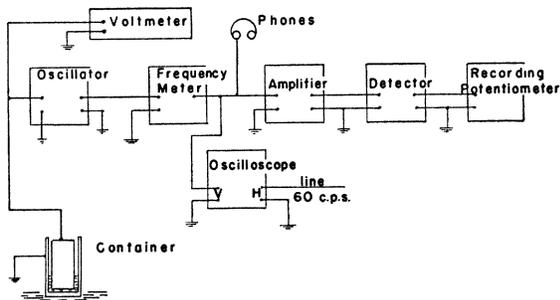
FIG. 2. Block diagram of the measuring circuits.
