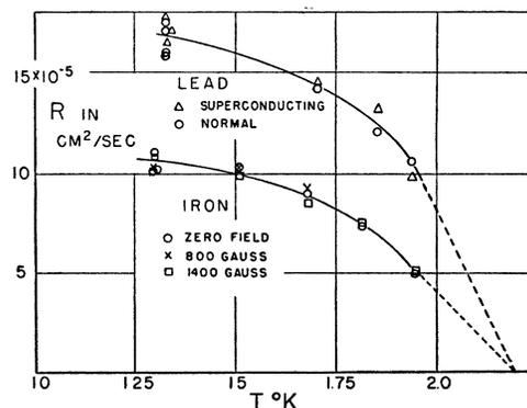
FIG. 10. HeII film transport rates over lead and iron.
