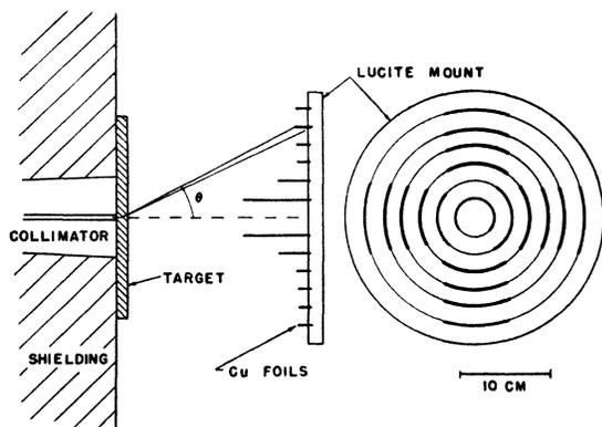
FIG. 1. Experimental arrangement.
