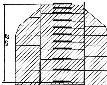
FIG. 1. Lead absorber.
