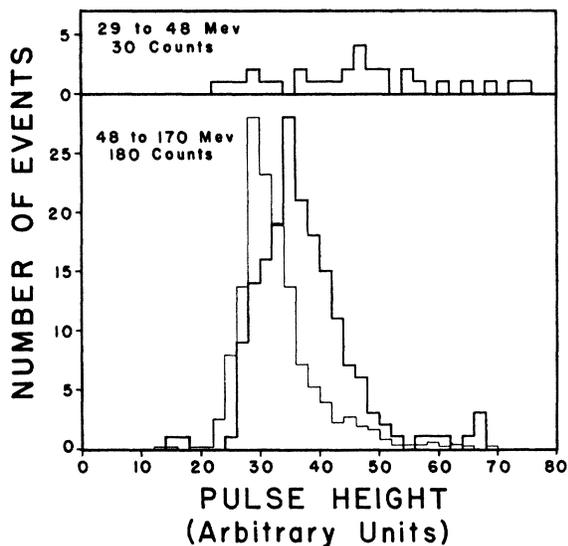
FIG. 2. Upper histogram: the distribution of pulse heights for  $\mu$ -mesons of energies between 29 and 48 Mev [range (a)]. Lower histogram: the heavy curve shows the distribution of pulse heights for meson energies between 48 and 170 Mev [range (b)]. The light curve is the distribution of Fig. 1A, which is shown for comparison.
