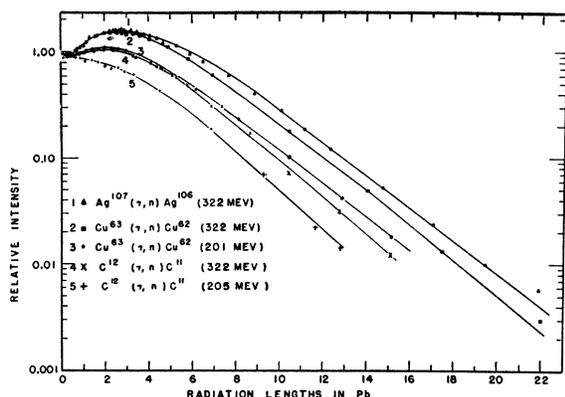
Fig. 4. Semilogarithmic plot of transition curves of x-rays responsible for several  $(\gamma, n)$  reactions.
