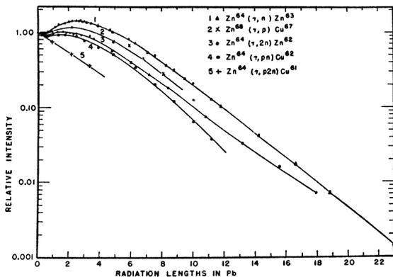
Fig. 5. Semilogarithmic plot of transition curves of x-rays responsible for several reactions from Zn taken with 322-Mev bremsstrahlung.
