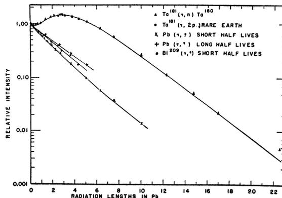
FIG. 6. Semilogarithmic plot of transition curves of x-rays responsible for several reactions from Ta, Pb, and Bi taken with 322-Mev bremsstrahlung.
