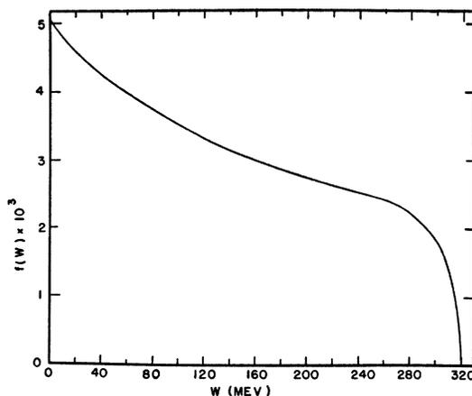
FIG. 7. Theoretical bremsstrahlung spectrum from the Berkeley synchrotron. The function  $f(W)$  is defined by Eq. (3). The ordinate scale is chosen to normalize the area under the curve to unity.
