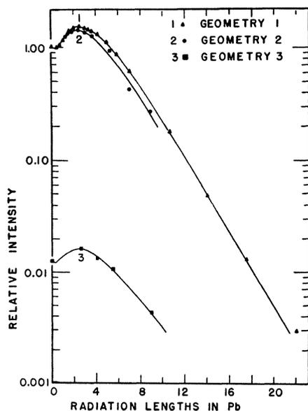
FIG. 2. Influence of geometry on transition curve in Pb of x-rays causing the reaction  $Cu^{68}(\gamma,n)Cu^{68}$ .
