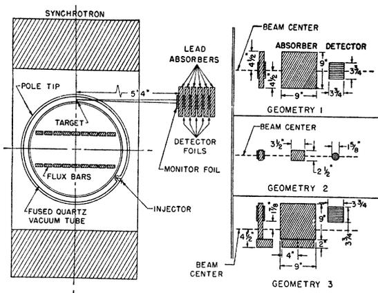
Fig. 1. Position of absorber stack with respect to the synchrotron and various geometries used in the experiment.
