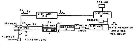
FIG. 1. Block diagram of electronics.
