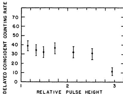
FIG. 2. Pulse 2B plateau. Plot of delayed coincidence counting rate against the relative height of a pulse required to make a delayed coincidence. Obtained by counting the number of delayed coincidences for different gain settings of amplifier 2B.
