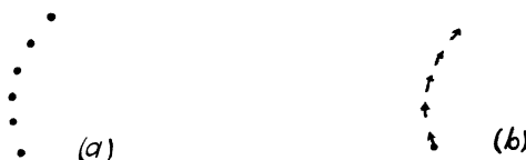
FIG. 2. Figure 2a shows a path defined by successive points and Fig. 2b shows the same path defined by successive tangents. Between two given points infinitesimally close to each other, the path followed by the particle is the classical path, i.e., a definite one; hence, it is possible to go from a point description to a tangent description of the path.
