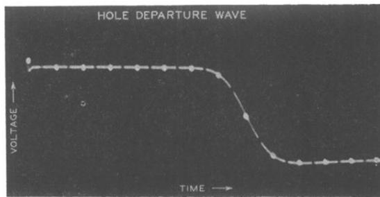
FIG. 3. Photograph of characteristic obtained on cathode-ray tube. Oscilloscope synchronized to stop of hole injection.
