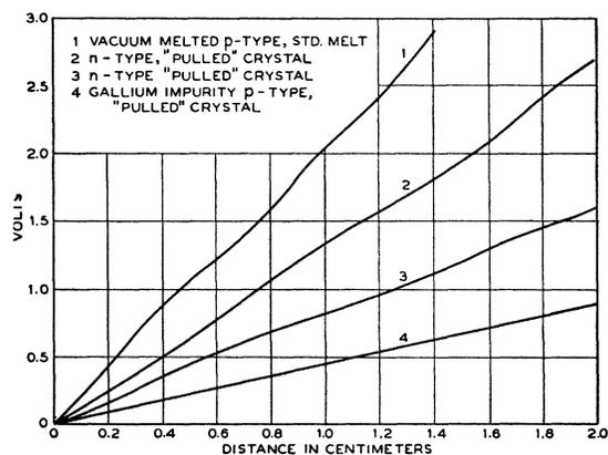
FIG. 5. Voltage as a function of distance along axes of typical samples for a current of 1.0 milliamperes.
