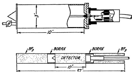
FIG. 1. Ionization chamber and arrangement of guard rings.
