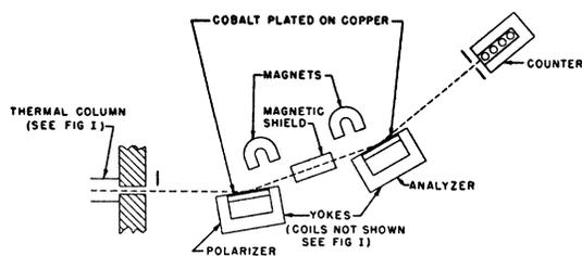
FIG. 8. Apparatus for the production of complete neutron polarization, and for measurement of polarization by the double reflection effect.
