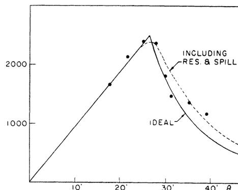
FIG. 3. Intensity of filtered neutrons reflected from a Be mirror as a function of incident angle,  $\theta$ . The solid line is a theoretical curve for infinite resolution and zero reflectivity above the critical angle, while the dashed curve includes corrections for finite resolution and partial reflectivity above the critical angle ("spill-over").
