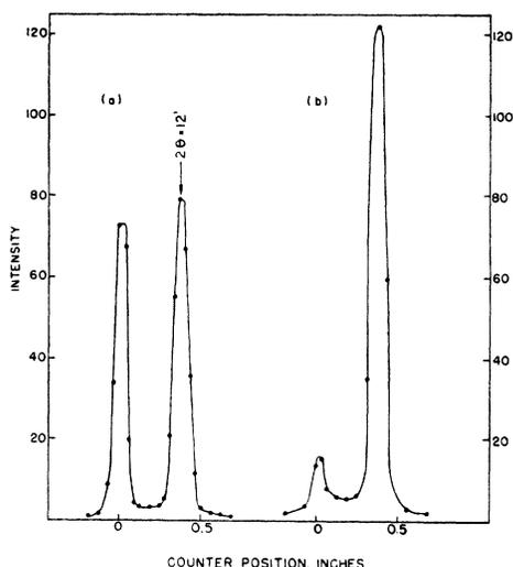
FIG. 2. Neutron beams observed with the apparatus of Fig. 1. The mirror intercepts about half the incident beam in (a) and almost the entire beam in (b). The direct beam is at the zero counter position while the reflected beam is at a position corresponding to a mirror angle,  $\theta$ , of 6 minutes.
