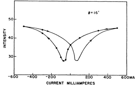
FIG. 5. Intensity of unfiltered neutrons reflected from a cobalt mirror as a function of magnetization.
