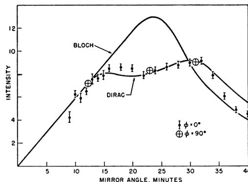
Fig. 4. Intensity of filtered neutrons reflected from a magnetized iron mirror. The theoretical curve labeled "Bloch" corresponds to Bloch's constant,  $C$  equal to zero, while "Dirac" corresponds to  $C=1$ . Experimental points for two directions of magnetization,  $\phi=0^\circ$  and  $90^\circ$ , are shown.
