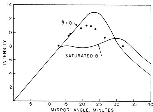
FIG. 6. Intensity of filtered neutrons reflected from an unmagnetized iron mirror as a function of incident angle,  $\theta$ . The curves are the expected intensities for two values of the effective magnetic field in the iron.
