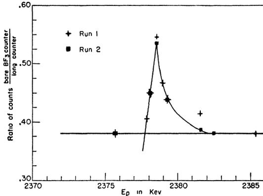
FIG. 1. Ratio of counts from a  $\text{BF}_3$  counter to those from a "long counter."
