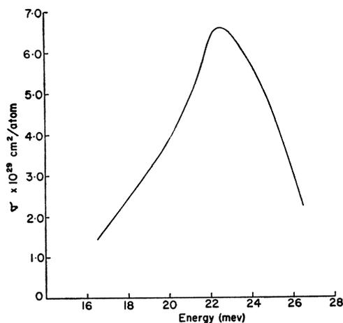
FIG. 2. Cross-section curve for the reaction  $\text{Rb}^{87}(\gamma, \alpha)\text{Br}^{83}$ .
