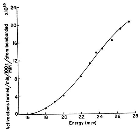
FIG. 1. Activation curve,  $\text{Rb}^{87}(\gamma, \alpha)\text{Br}^{83}$ .
