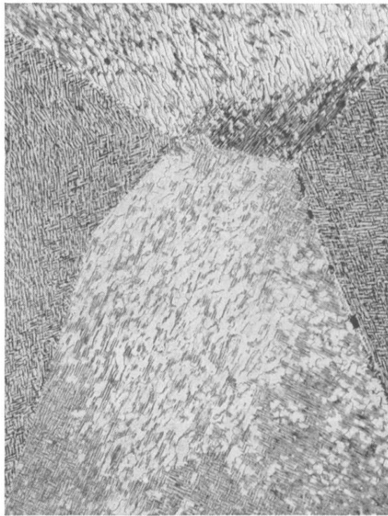
FIG. 2. Microstructure of Alnico 5 aged 300 hr at 800°C. X500.
