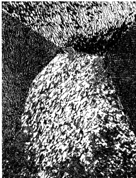
FIG. 2. Microstructure of Alnico 5 aged 300 hr at 800°C. \times 500 .
