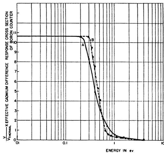
FIG. 7. Calculated effective *cadmium-difference* response cross section of a spherical and a parallel plate counter. Curve  $A$  is for the spherical counter, and curve  $B$  is for the parallel plate counter.
