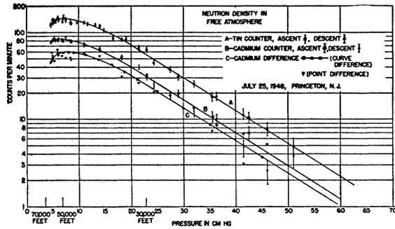
FIG. 5. Balloon flight made at geomagnetic latitude  $51^{\circ} 46'$  N on July 25, 1948, using a pair of  $\text{BF}_3$  counters (50 cm Hg pressure).
