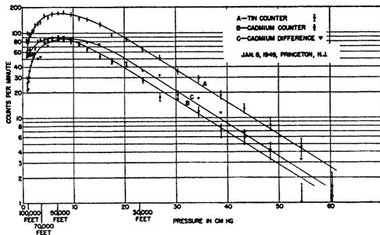
FIG. 6. Balloon flight made at geomagnetic latitude  $51^{\circ} 46'$  N on January 8, 1949, using a pair of  $\text{BF}_3$  counters (50 cm Hg pressure).
