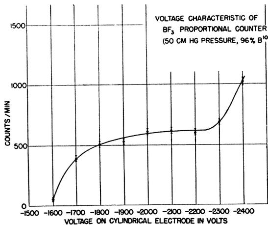
FIG. 1. Voltage plateau characteristic of proportional counter.
