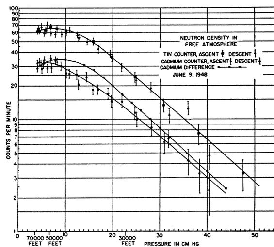
FIG. 4. Balloon flight made at geomagnetic latitude 51° 46' N on June 9, 1948, using a pair BF<sub>3</sub> counters (20 cm Hg pressure).
