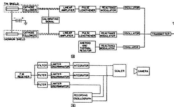
FIG. 2. Block diagram of telemetering and receiver system.
