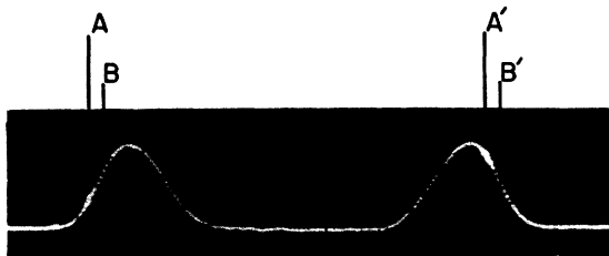
FIG. 8. Photograph of a typical cyclotron resonance trace at the 9th multiple of \nu_R . The vertical deflection is proportional to the detector probe current; in the horizontal direction, the dee frequency first increases and then decreases, thus sweeping twice through resonance. The two bright spots on the trace at A and A' are the frequency markers, which are slightly displaced from their true positions B and B' because of time delay in the amplifiers. The relative width at half maximum amplitude is about 1/9000 for this resonance curve.
