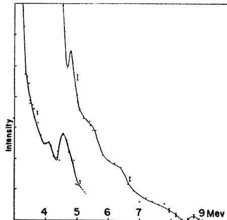
FIG. 3. Neutron capture  $\gamma$ -ray spectrum from cadmium.
