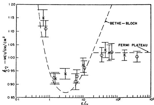
FIG. 2. Dashed curves show Bethe-Bloch energy loss, and Fermi plateau for AgBr. Experimental points, with standard deviations indicated; ○— $\mu$ -meson decay electrons, and relativistic  $\mu$ -mesons in sea-level plate; ×—high energy electrons, protons, and shower  $\pi$ -mesons in high altitude plate.
