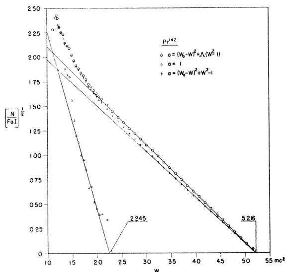
FIG. 5. The modified Kurie plots of  $\text{Pr}^{142}$ . The low energy group was obtained by the usual subtraction.
