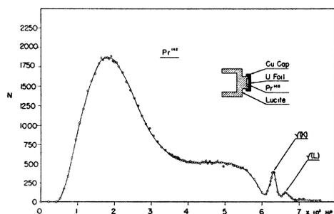
FIG. 1. Secondary electron distribution produced by Pr<sup>142</sup>, from a copper cap (1.4 g/cm<sup>2</sup>) and a uranium foil (42 mg/cm<sup>2</sup>). The insert shows the Lucite holder, Pr<sup>142</sup>, copper cap, and uranium foil. *N* is the observed counting rate. This diagram shows the electron distributions produced by bremsstrahlung, Compton scattering and the photoelectric effect.
