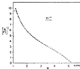
FIG. 4. The allowed Kurie plot of the beta-spectrum of  $\text{Pr}^{142}$ .
