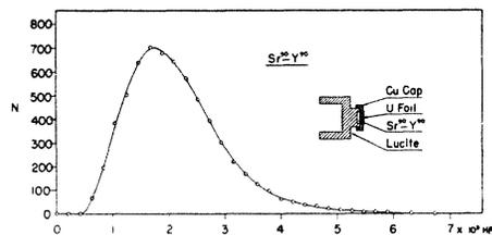
FIG. 2. Secondary electron distribution produced by a pure beta-source of  $\text{Sr}^{90}\text{-Y}^{90}$ , from a copper cap ( $1.4 \text{ g/cm}^2$ ) and a uranium foil ( $42 \text{ mg/cm}^2$ ). The electron distribution is produced by the bremsstrahlung formed in the copper cap due to the absorption of the beta-rays from  $\text{Sr}^{90}\text{-Y}^{90}$ .
