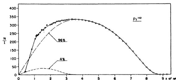
FIG. 3. Beta-spectra of  $\text{Pr}^{142}$ . The solid curve is the observed spectrum while the dashed curves represent the two beta-groups, calculated from the respective Kurie plots.  $N$  is the observed counting rate and  $I$  is the current in the spectrometer coil.
