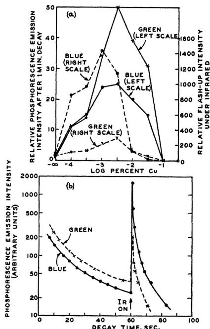
FIG. 1. (a) Phosphorescence emission intensity at room temperature after one minute decay, and flash-up intensity under infra-red stimulation as a function of copper proportion in hex.—ZnS:Cu(0.0–0.3), [NaCl(2)] phosphors. (b) Phosphorescence emission decay at room temperature before and during infra-red illumination for hex.—ZnS:Cu(0.001), [NaCl(2)].
