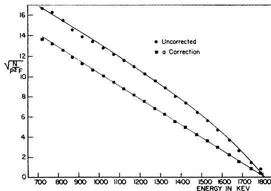
FIG. 2. Fermi plots for Rb<sup>86</sup> high energy spectrum.
