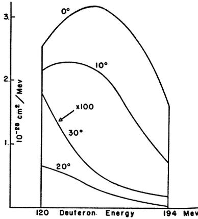
FIG. 5. Spectrum at various angles of the deuterons produced by 200-Mev nucleons.
