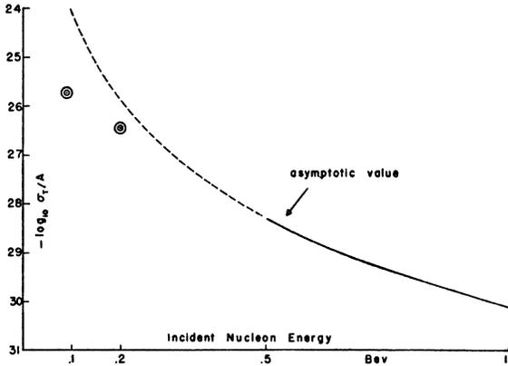
FIG. 6. Total cross section for production of deuterons as a function of the incident nucleon energy.
