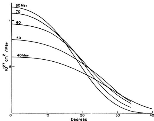
FIG. 3. Differential cross section per Mev and per nucleon for production of deuterons by 90-Mev nucleons.
