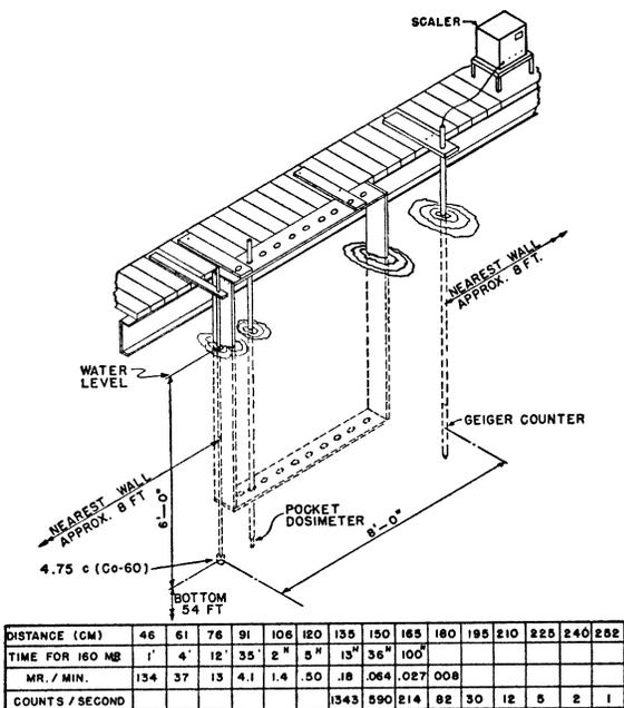
FIG. 1. Experimental arrangement.
