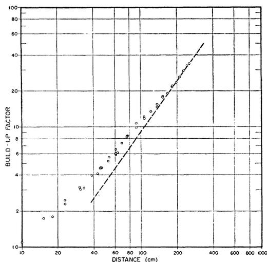
FIG. 3. Logarithmic variation of build-up factor with distance.
