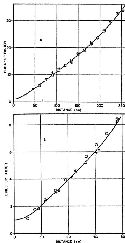
FIG. 2. The build-up factor as a function of distance. (A) Data from the present experiment. (B) Collection of data from various experiments for moderate penetration. + NBS, 0.33 curies, ionization data; □ NBS, 4.75 curies, ionization data; ⊙ NBS, 4.75 curies, counter data; ○ NRL, 0.04 millicurie, counter data; △ MIT, 1.9 curies, ionization data.
