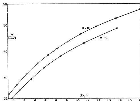
FIG. 5. Slowing-down density exponent as in Eq. (47') for  $M=\infty$  and  $M=9$  for larger  $z/u'$ .
