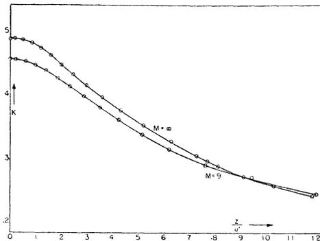
FIG. 3. Slowing-down density coefficient in Eq. (47) for  $M = \infty$  and  $M = 9$ .
