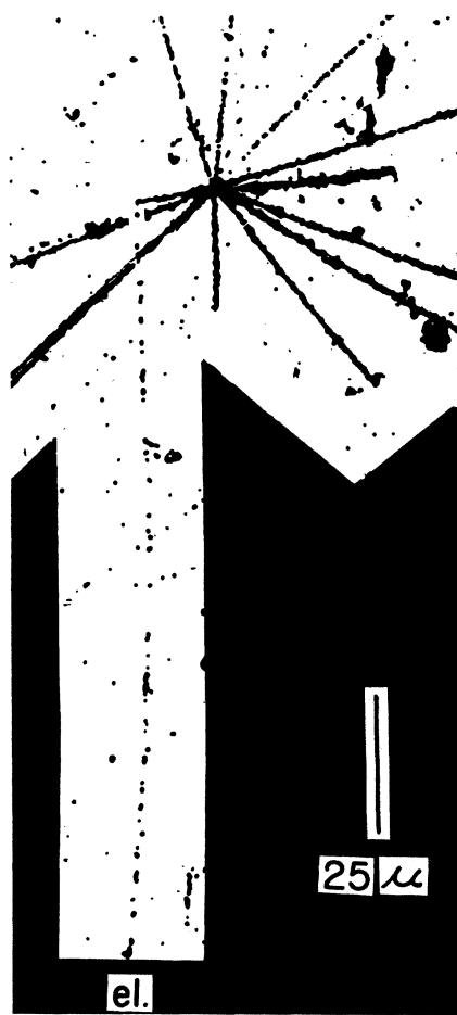
FIG. 1. Fifteen-pronged star with nucleus, from the end of which originates a decay electron.
