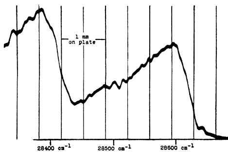
FIG. 4. Microphotometer trace of the (1, 6) band of O_2^+ at 3494A. The slit was opened to produce a line width of 30\text{ cm}^{-1} . Both first and second band heads are shown. After intensity calibration this band shape is related to rotational temperature in Fig. 5.
