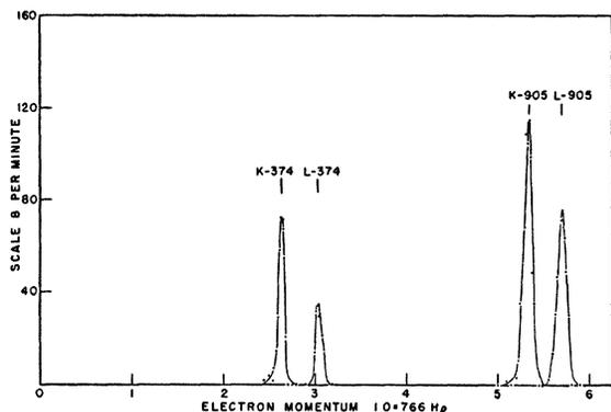
FIG. 1. Spectrum of internal conversion electrons from  $Pb^{204m}$ .
