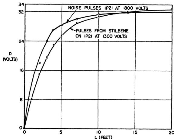
FIG. 1. Rise of noise pulses and pulses from stilbene. D is the discriminator reading corresponding to a constant counting rate. L is the length of shorted delay cable (4 feet of which correspond to a time delay of  $10^{-8}$  sec.).
