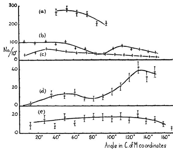
FIG. 1. Angular distribution of protons from the reaction  $B(\alpha, p)C^*$ .
