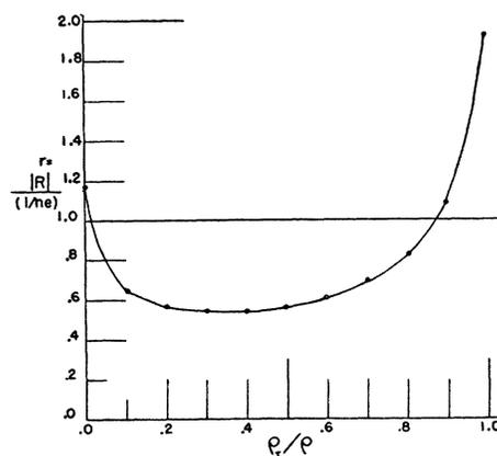
FIG. 1. The dependence of  $r = |R|/(1/ne)$  on the ratio of  $\rho_I$ , resistivity due to Rutherford-type scattering by impurity ions, to  $\rho$ , the total resistivity.
