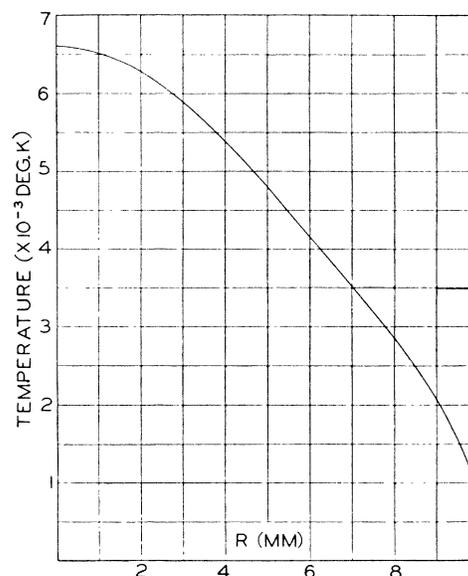
FIG. 1. Temperature distribution in the Hg arc.
