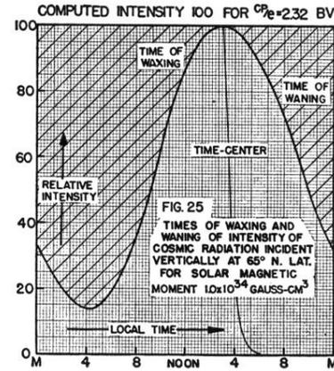
Figs. 20-25. Samples of the third graphical step in the derivation of the diurnal variation from the deflection curves.
