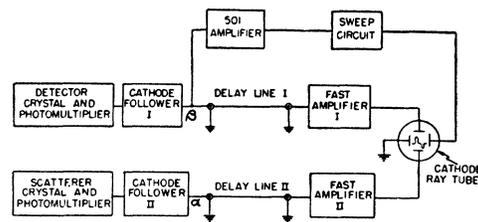
Fig. 3. Block diagram of scheme for detecting small time differences.
