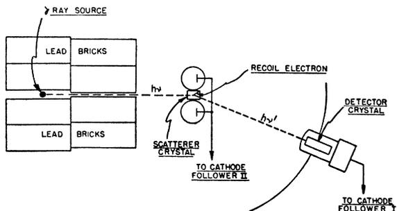
FIG. 1. Sketch of Compton scattering apparatus.
