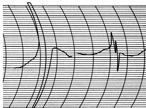
FIG. 6. Automatic recording tracings of J=19 \rightarrow 20 , \Delta F = +1 transitions of ICN at \lambda = 2.32 \text{ mm} obtained by use of phase sensitive amplifier with source modulation. Left curve shows unresolved line. Right curve is partially resolved. The presentation represents the first derivative of the absorption curve.
