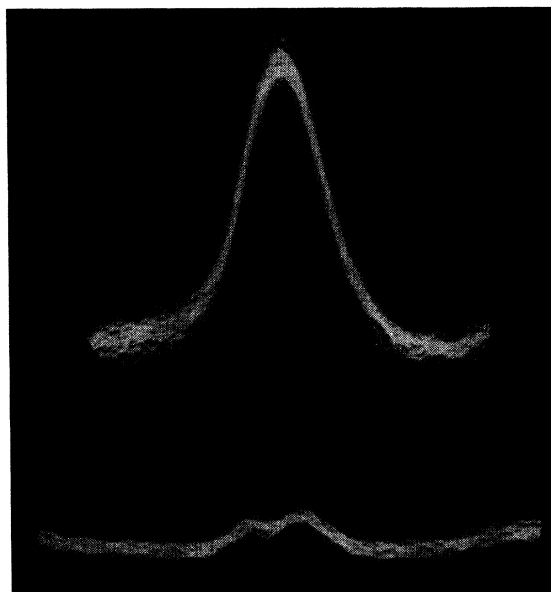
FIG. 4. Upper curve shows the unresolved J=19 \rightarrow 20 , \Delta F = +1 transitions of ICN at \lambda = 2.32 mm. Lower curve shows the same transition partially resolved.
