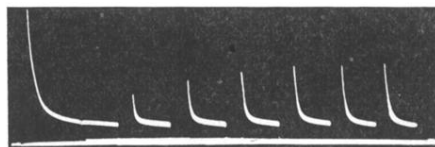
FIG. 13. Release of trapped electrons. Initial pulse length = 6 \mu\text{sec} . Test pulse length = 4 \mu\text{sec} . at 5 \mu\text{sec} . intervals.
